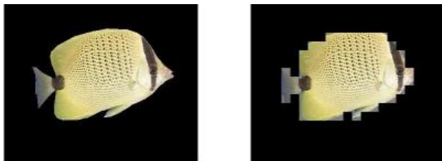
Fig. 1. Alpha threshold influence on the VOP visual quality: left - alpha\_th=0 ; right - alpha\_th=256
